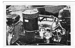
Two views of the power unit showing (left) disposition of the magneto, carburetters, airstlencer, cut-out, fuse-box and so on. (Right) The 12-volt battery is accessibly mounted in the insulated bulk-
