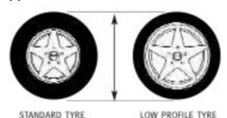
The rim diameter may be varied from the standard size but the overall diameter of the tyre must not vary by more than +15mm or -26mm.
