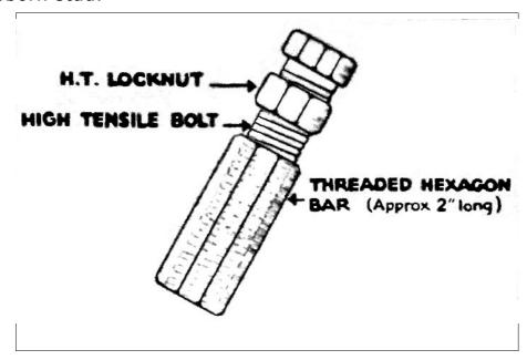
It's a good idea to have a set of these stud boxes made up in sizes to suit your car—head and manifold studs are the most common requiring removal. (A. E. Hodges, Malvern, Vic.)
