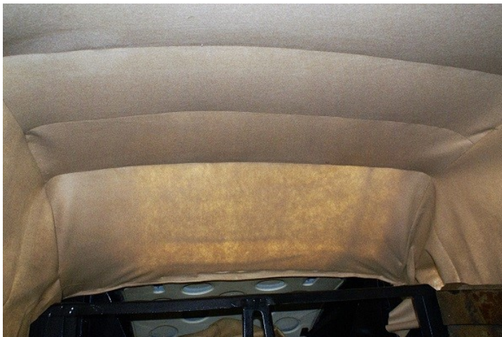
Above: The rear of the headlining. From this picture you can see that the rear corner sides need to be adjusted further.
