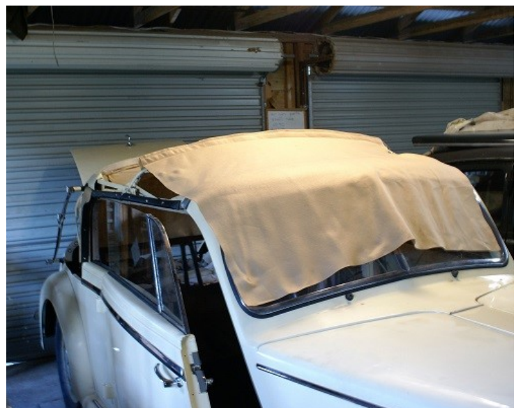
Above: The headlining draped for further measuring.
