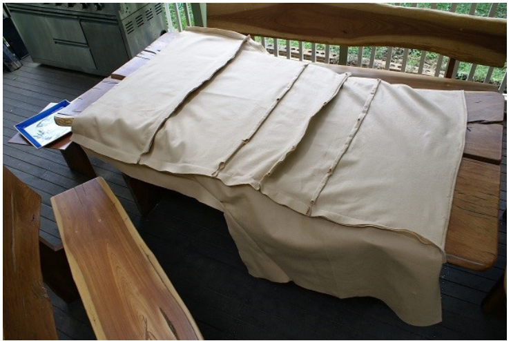
Pictured above: The headlining roughly set out with loops or sleeves for the rods and the cut outs for the screws
