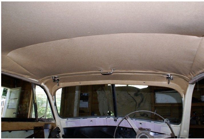
Above: The headlining is a bit loose on the drivers side and not pulled over to the passenger side sufficiently. Small but necessary corrections.
