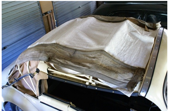
Above: The headlining is a bit loose on the drivers side and not pulled over to the passenger side sufficiently. Small but necessary corrections.
