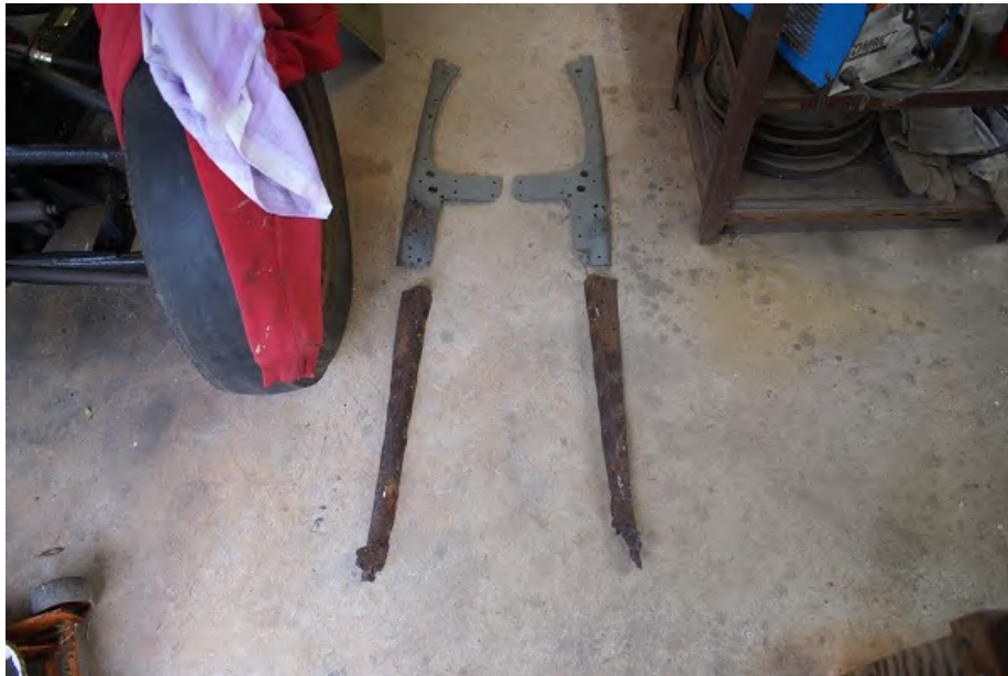
Original reinforcing steels for bottom and top of the 'A' post.
