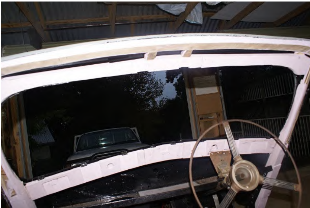
Header stick, top window surround and door posts fitted.
