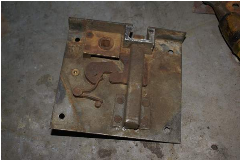
and Ross' passenger door lock working parts
