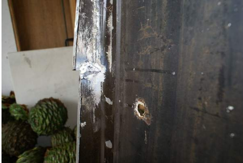
Weld over the stress fracture
