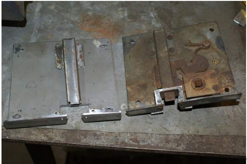
Door lock housing, lock bolt and spring
